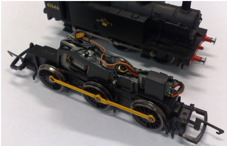
Figure 2: Model railway locomotive showing a small electronic circuit that implements a “DCC decoder” using an ultramicrocontroller.
