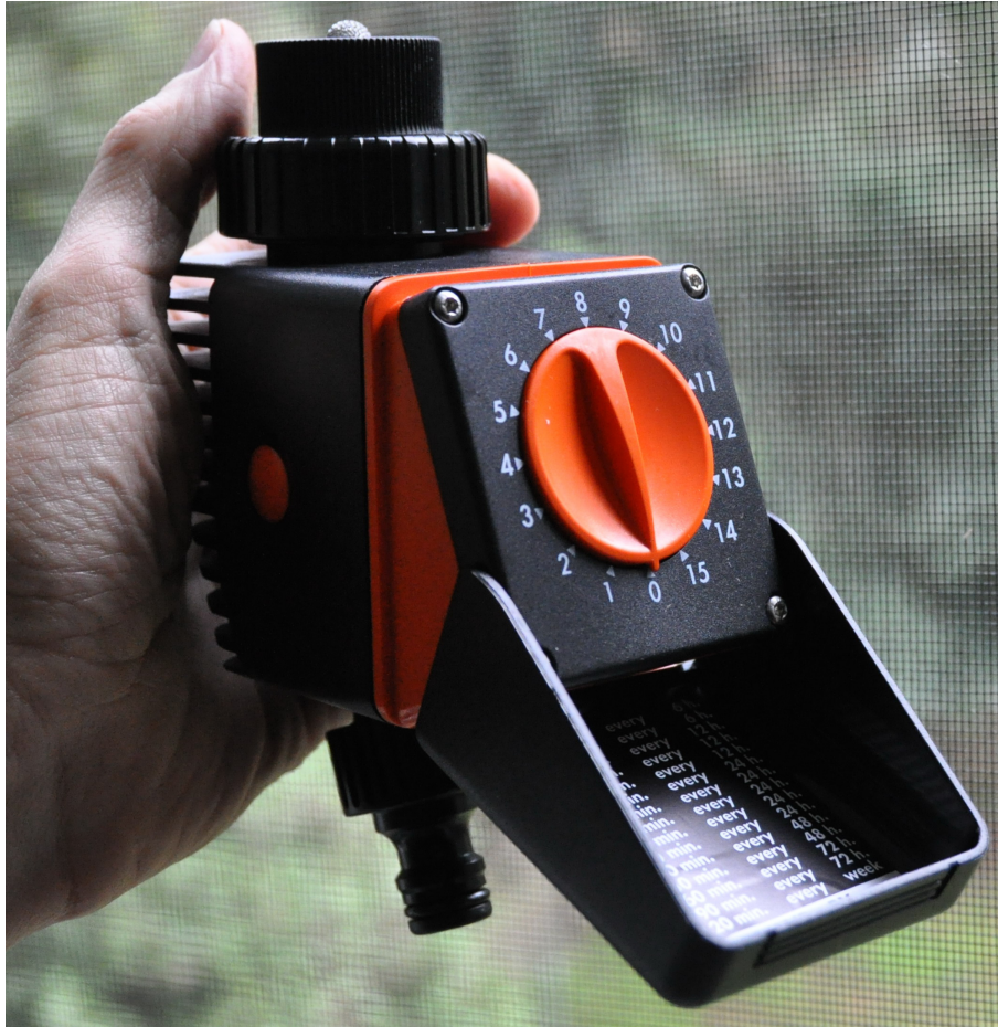
Figure 1: Example of a garden tap timer. One (in this case) or two knobs set the frequency and duration for which the timer turns on the water flow. Devices typically operate for a year on a battery.
